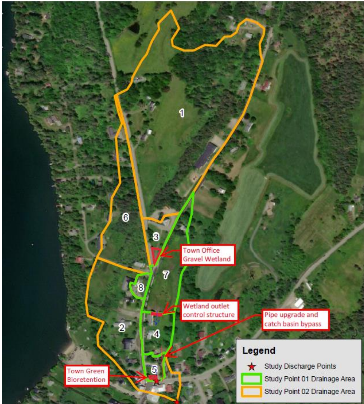
Figure 3. Project drainage area with proposed BMPs in red. Additional grading and infrastructural upgrades that are not pictured here accompany some designs. More information can be found on the design drawings.
